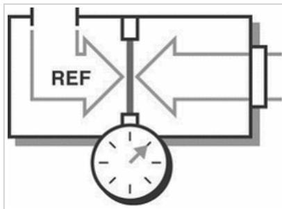
Gauge pressure is measured relative to ambient atmospheric pressure (see picture). Similar to absolute pressure, the abbreviations PAG (Pascals Gauge) or PSIG (Pounds per Square Inch Gauge) are used to describe gauge pressure.
