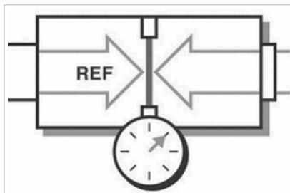
Differential pressure is similar to gauge pressure, but instead of measuring relative to ambient atmospheric pressure, differential measurements are taken with respect to a specific reference pressure (see left). Also, the abbreviations PAD (Pascals Differential) or PSID (Pounds per Square Inch Differential) are used to describe differential pressure.
